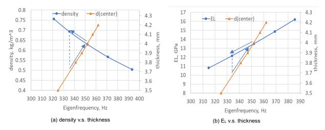
Fig.8 Change of mode 5 eigenfrequency and relation between thickness  $d_{(center)}$ , density and elasticity.
