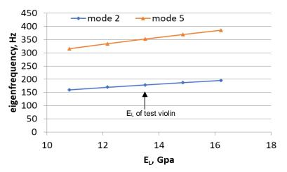
Fig.6 Change of eigenfrequencies by the difference in  $E_{\rm L}$  of back-plate.
