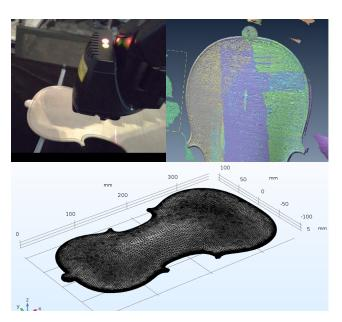
Fig.1 Snapshots scanning the surface of violin back plate (upper row, left), revising the geometry (upper row, right) and importing the mesh data to COMSOL Multiphysics (lower row).
