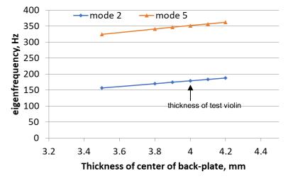
Fig.5 Change of eigenfrequency by the change in thickness of back plate. The thickness in horizontal axis is the thickest point in the center of back plate. 4.0 mm is the thickness of test violin used in this study.
