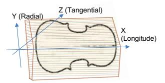
Fig.2 Orthotropic property of violin plate. Because wood is orthotropic material, we set the typical (or real) value of orthotropic properties of the wood to the parameters of COMSOL Multiphysics.
