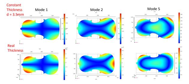
Fig.3 Mode shapes of back-plate of violin, (a) mode 2 (x-mode), (b) mode 5 (ring mode).
