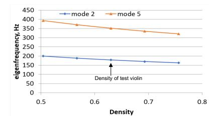
Fig.7 Change of eigenfrequencies by the difference in density of back-plate.
